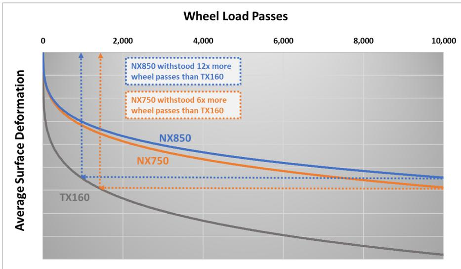
**Figure 9.** Aggregate surface deformation results for NX850, NX750 and TX160 sections.
