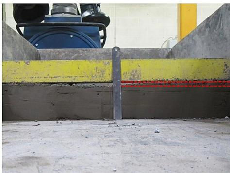
**Figure 8.** Enlarged photo of the subgrade rutting in the NX850 section. The minimal amount of rutting experienced is noted by the red dashed lines.
