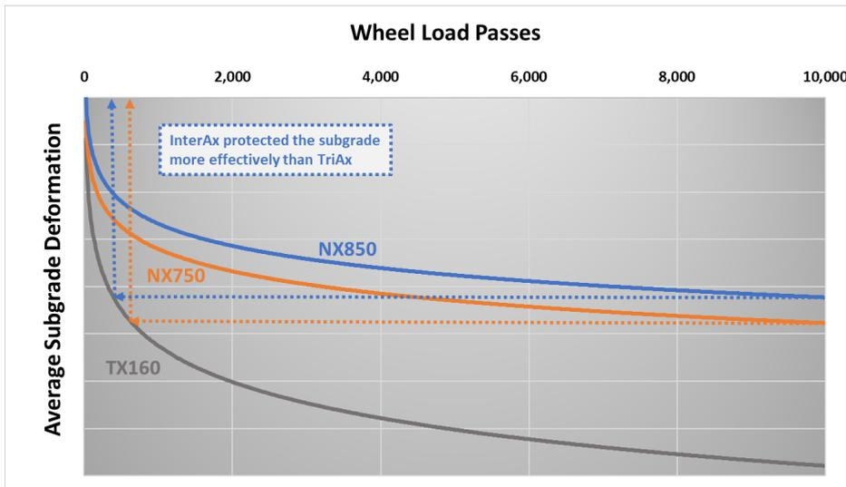
**Figure 10.** Subgrade deformation results for NX850, NX750 and TX160 sections.
