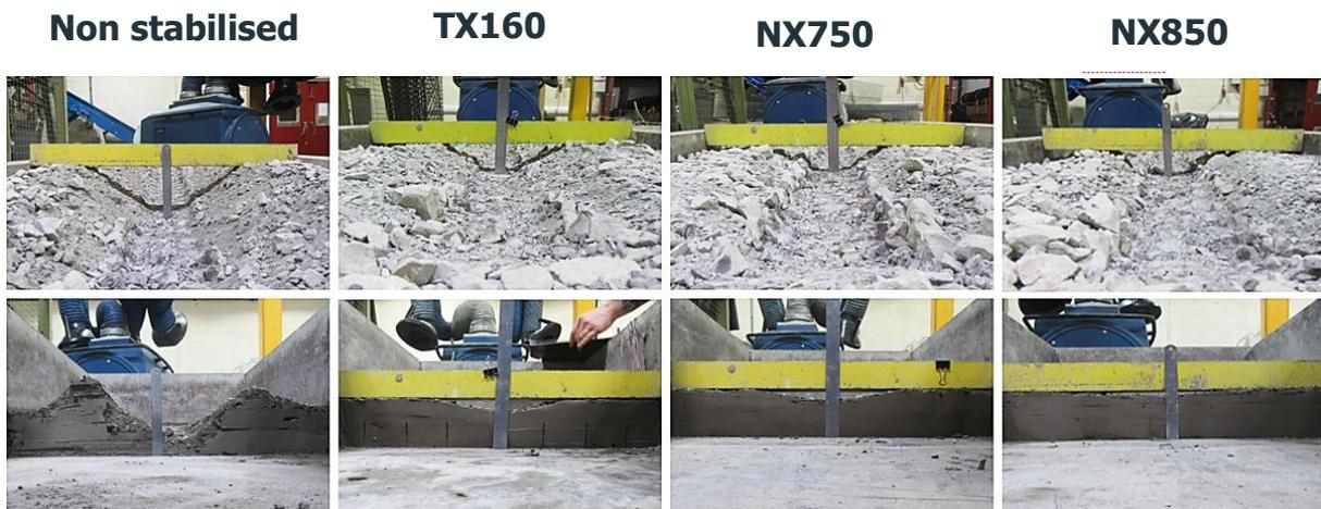
**Figure 7.** Aggregate surface (top photos) and subgrade (bottom photos) rutting profiles after trafficking. The yellow straight edge is used to improve visual comparison of the sections. InterAx NX850 experienced the least surface and subgrade rutting.
