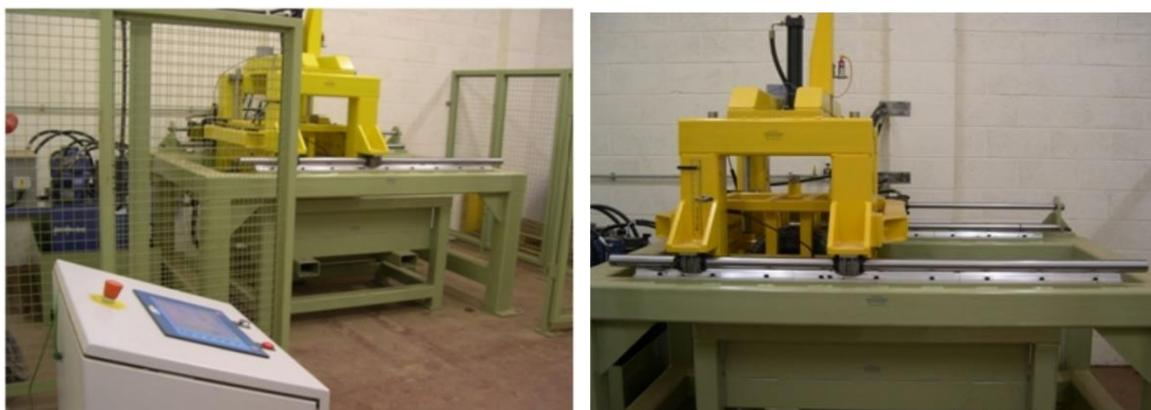
**Figure 4.** The trafficking device, associated controls, and test box.
