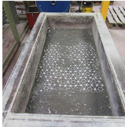
**Figure 6.** The NX750 exhumed after trafficking is complete.
