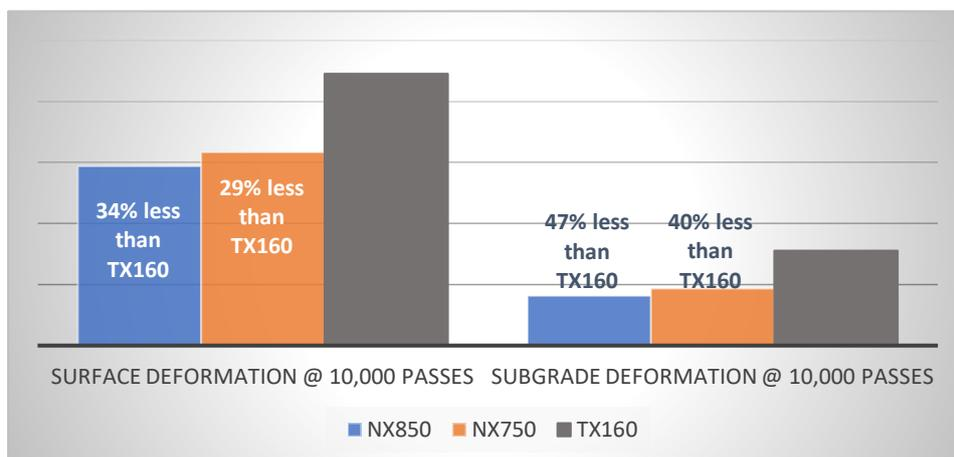
**Figure 11.** Surface deformation and subgrade deformation of NX850 and NX750 compared to TX160, after 10,000 passes of the wheel load.
