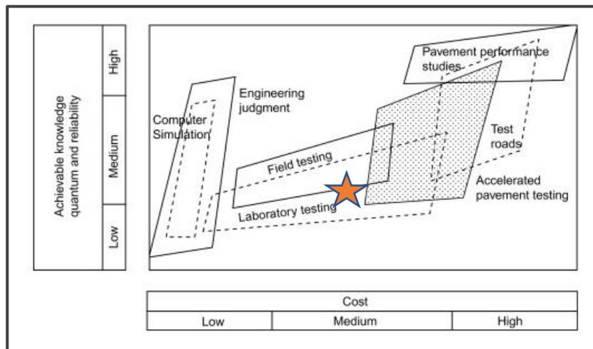
**Figure 3.** Relationship between pavement engineering test types (reliability and knowledge gained) and cost (from Hugo et al. 1991.). The relative location of this research report is indicated by a star on the chart.
