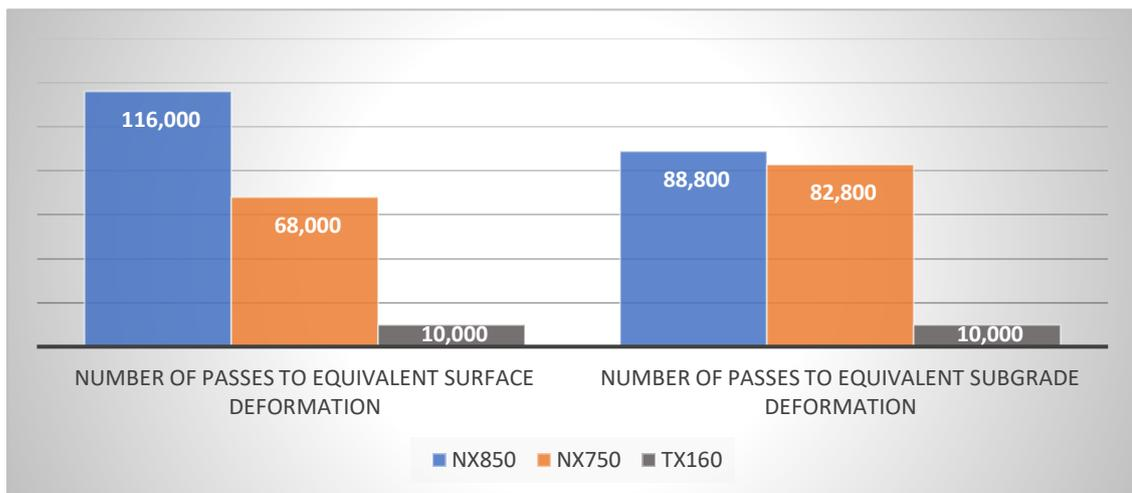
**Figure 2.** Number of passes for NX850 and NX750 to achieve equal surface and subgrade deformation to TX160, based on power model.
