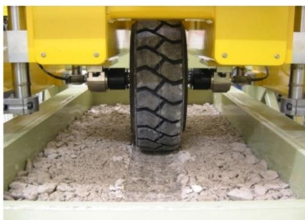
**Figure 5.** The trafficking device in service. The pressure applied is approximately 600 kPa, which is equivalent to a conventional, fully loaded truck tire.
