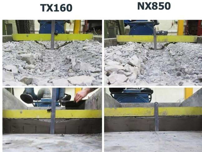
**Figure 1.** Aggregate surface (top photos) and subgrade (bottom photos) rutting profiles after trafficking.
